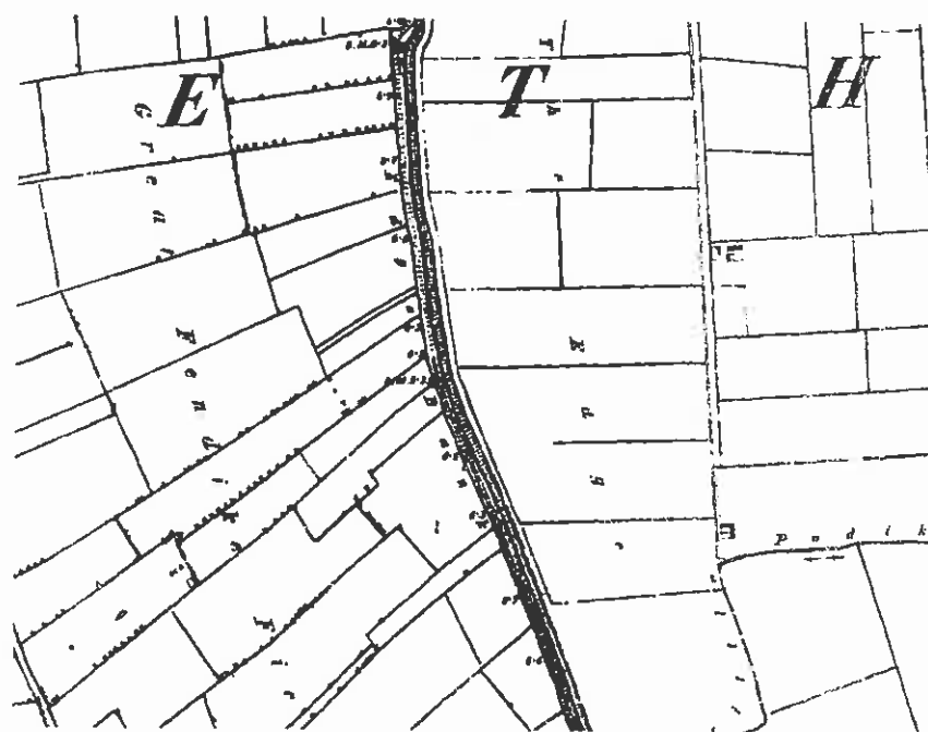
Figure 2: the junction of anciently-drained fen (left), with characteristic sinuous dyke pattern; and more recently enclosed, and more rectilinear, fen (right).
